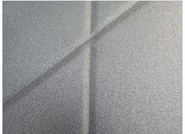
NARROW-ROLLER LEAF EMBOSSING TECHNOLOGY CROSS LINE
